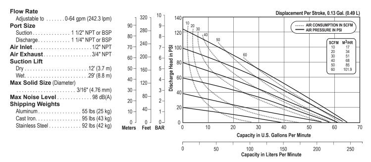
NOTE: Performance based on the following: PTFE fitted pump, flooded suction, water at ambient conditions. The use of other materials and varying hydraulic conditions may result in deviations in excess of 5%.
