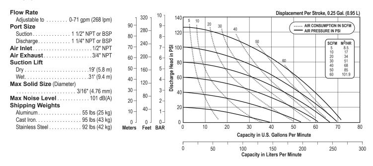
NOTE: Performance based on the following: elastomeric fitted pump, flooded suction, water at ambient conditions. The use of other materials and varying hydraulic conditions may result in deviations in excess of 5%.
