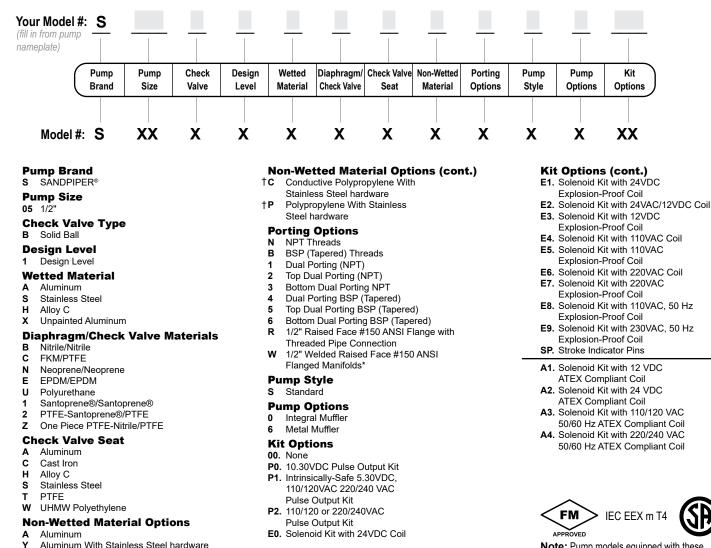
+ Note: Pumps equipped with non-wetted options C or P are limited to a maximum operating pressure of 100 psi or 7 bar.
